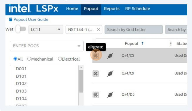
12 Confirm that an Airgrate will be installed for this Popout.
